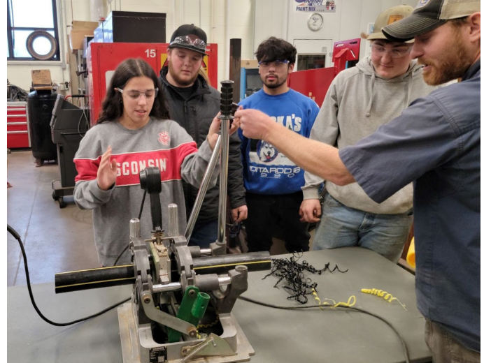
Josh Fenske, Northcentral Technical College Gas Utility Construction Instructor, teaches East High Tech Ed students how to fuse utility line pipes together. As of February 2023 East High has two senior students signed up for NTC's Gas Utility Construction Program.
